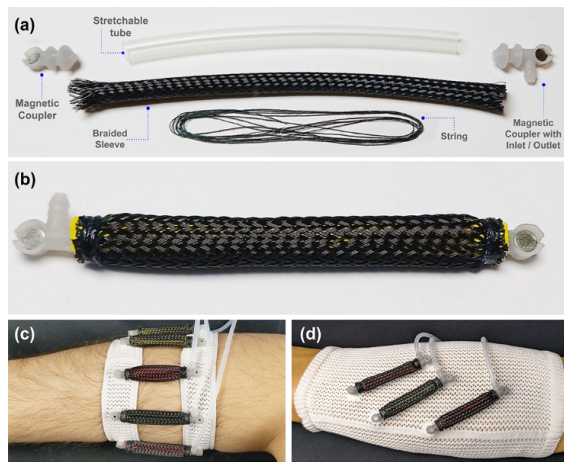
Figure 11: A muscle module (a) before assembly and (b) after assembly. (c, d) The modules can be attached to the sleeve in any orientation or configuration.
