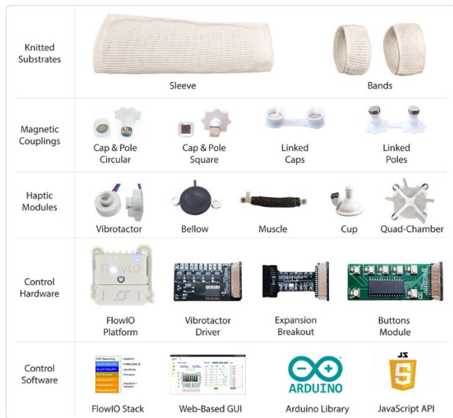
Figure 2: The complete SleeveIO toolkit consisting of Knitted Substrates, Magnetic Couplings, Plug-and-Play Modules, Control Hardware, Control Software with APIs and a GUI.
