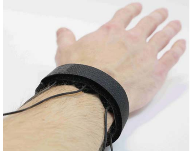
Fig. 1: Bellowband is a pneumatic wristband that can deliver local pressure and vibration at eight positions around the wrist. The device is made from thermoplastic polyurethane (TPU), resulting in a lightweight wristband capable of rendering complex pressure and vibration to the user.
